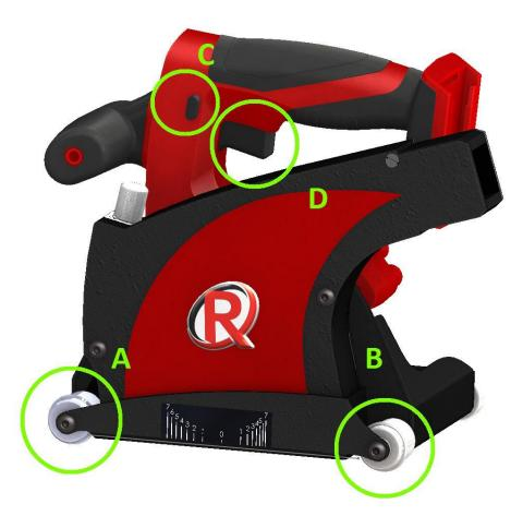
Lower the handle slowly until it is in the stop. Maintain this position and then move the grooving machine along the joint. After a few centimetres, the rear guide caster (wider) penetrates directly into the chamfer created already, finally providing guidance for the machine.
