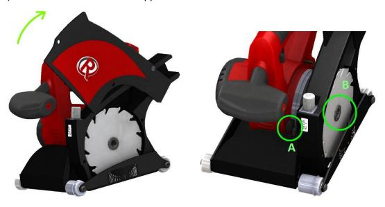
Remove the pin, then the worn blade and replace it, paying attention to the direction of rotation
